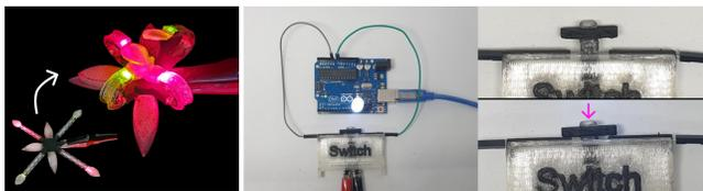
**Figure 24: Discrete LEDs integrated in a shape-changing flower mood light (left), and a switch mechanism integrated with a micro-controller (right)**
