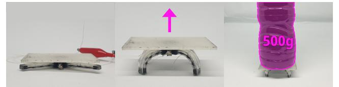
**Figure 22:** Self-standing table that bears 500g after its shape-transformation
