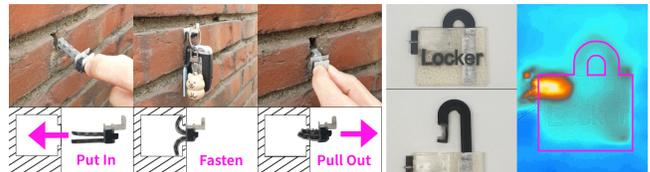
Figure 23: A fastener actuates *inside a wall*, where it is not reachable (left). Actuating the inner (unreachable) mechanism of a lock (right)
