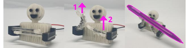
**Figure 21:** Sequentially unfolding the two arms to avoid self-collisions
