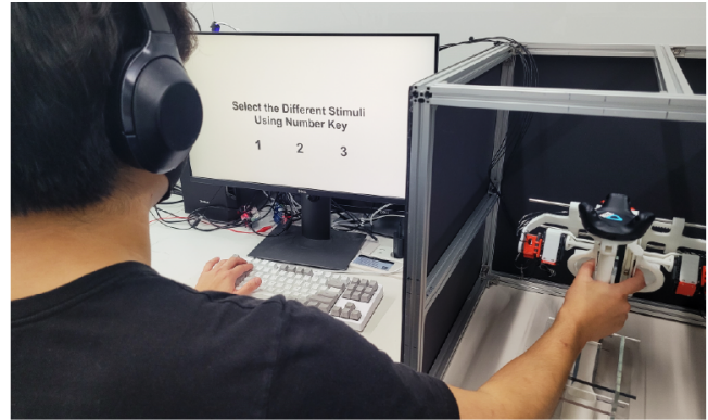
Figure 7: The JND study setup. Participants listened to white-noise through headphones as they experienced skin-slip feedback with their dominant hand and input their response with their other hand through keyboard input.
