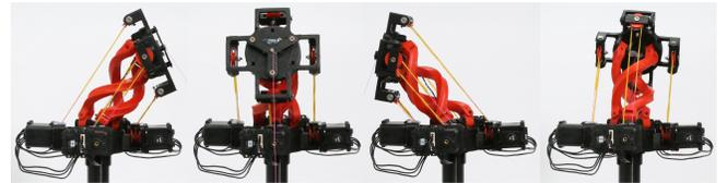
Figure 4. The quaternion joint achieves 2-DOF wide rotational angle.
