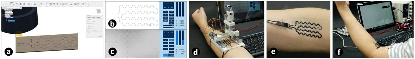
**Figure 2. BodyPrinter's workflow.** (a) Generating a G-code file. (b) Loading the G-code in the BodyPrinter's software, making changes on the fly, setting parameters, and (c) calibrating. (d) Printing the sensor. (e) Applying other electronic components on the sensor, and (f) demonstrating its usage.
