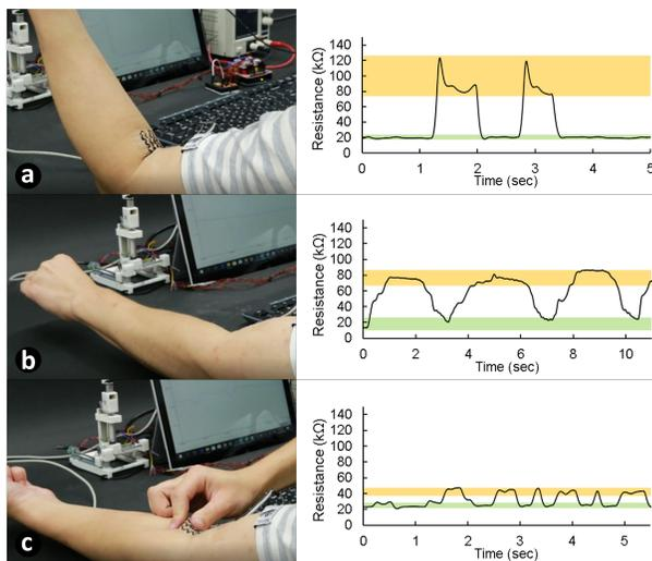
**Figure 10.** The images of 3 input postures (bending (a), twisting (b), squeezing (c)) and their measured resistance over time. The range of resistance for the idle and input postures are highlighted in green and yellow respectively.
