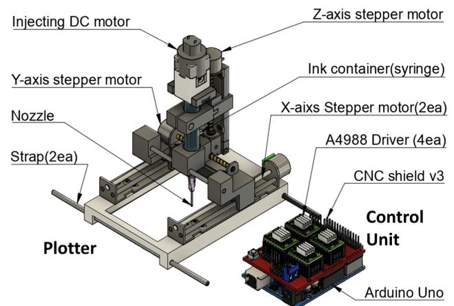
**Figure 3. Isometric view of BodyPrinter structure and its parts.**
