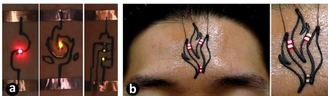
**Figure 11.** Various examples of LED displays printed on the arms (a) and on the forehead (b). The latter shows a charlieplexing configuration, with six LEDs individually controlled using only three wires.
