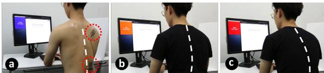
**Figure 7.** A pair of strain gauge sensors placed on the back are used to sense good (a), moderate (b), and bad (c) postures.
