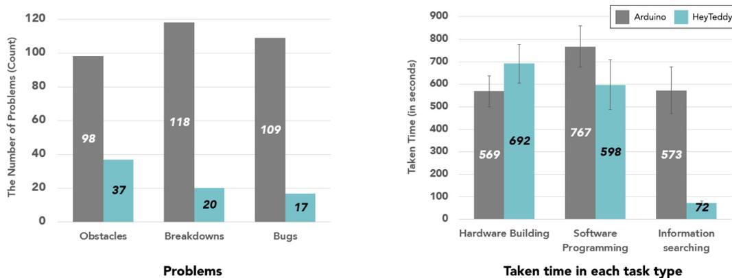
Fig. 8. Performance of HeyTeddy vs Arduino for number of problems (left), and task times (right).
