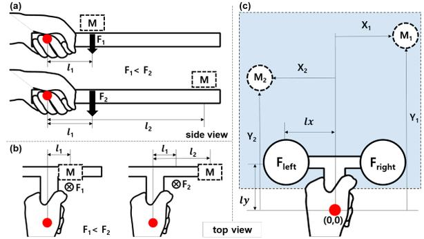
**Figure 2.** Our device creates the illusion of a shifting weight because (a,b) the thrust of its two propellers generates a force that pivots the device's handle around the user's wrist. Moreover, (c) by modulating the speed of these propellers, it can mimic a weight shift on two dimensional plane (as illustrated by the X,Y coordinates above).
