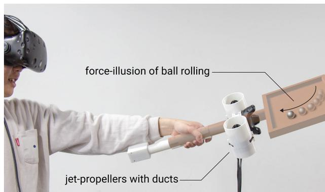
**Figure 1.** *Aero-plane* is a handheld device capable of emulating a shifting center of mass in 2 degrees-of-freedom by driving two jet-propellers to generate dynamic force-feedback. Here, we demonstrate our device rendering the weight of a virtual ball as it rolls on a virtual box that the user is interacting with.
