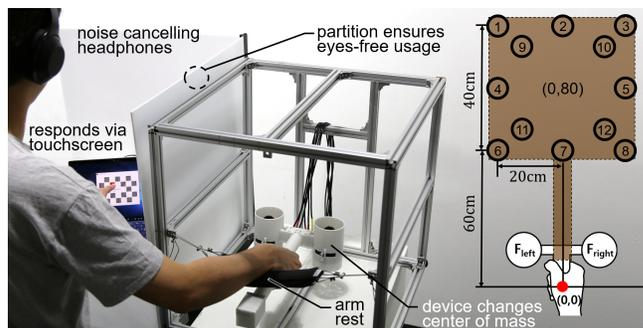
Figure 9. Setup for our user study: participants sat down, without visual contact with the device, and felt the pulling force of the device on their dominant hand. Then, participants used a touchscreen with their non-dominant hand to indicate the perceived weight movement.
