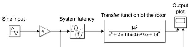
Figure 7. Simulink setup
