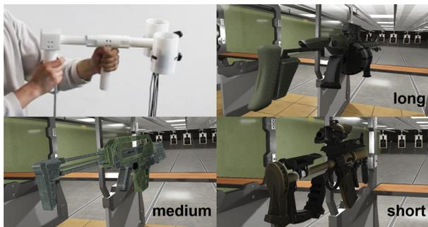
Figure 15. Gun VR application: User shown holding the device with a gun handle shaped attachment and wearing a HMD (top left). Different haptic feedback is given to the user corresponding to the length of the gun, and muzzle rise feedback is given while the trigger is pressed.
