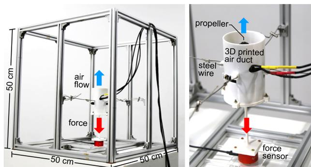
Figure 4. Our measurement setup (left). Close-up of how the propeller pulls on the force sensor (right).
