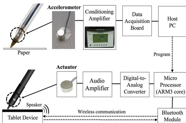
Figure 6. Hardware of RealPen setup.
