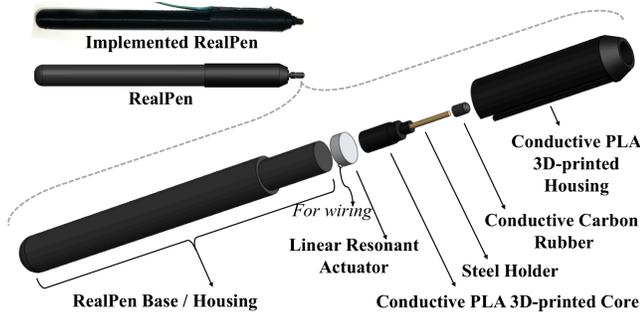
Figure 3. Implemented RealPen and its schematic illustration.
