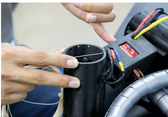
→ Weaving a tennis string net on the air ducts for safety.
