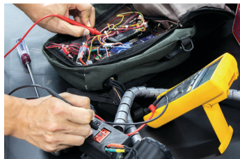
→ Debugging the electronic components before final assembly.
